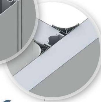
Site assembled 3-way corner detail
